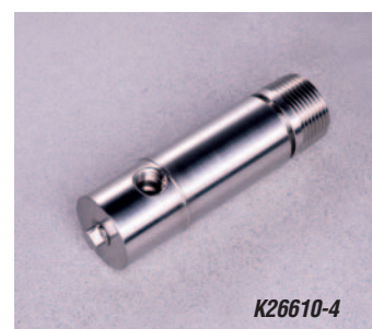
Flow-through design with 1/4" NPTF thread, flow rates to 1/2 lpm, jacketed for temperature control.
